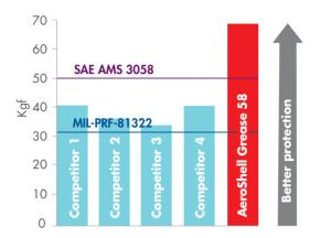
A step change in extreme-pressure protection. AeroShell Grease 58 has **better load wear protection** compared with MIL-PRF-81322 greases in ASTM D2596 tests.
