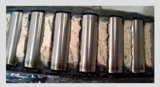
AeroShell Grease 58, which meets the SAE AMS 3058 specification, after 548 cycles
